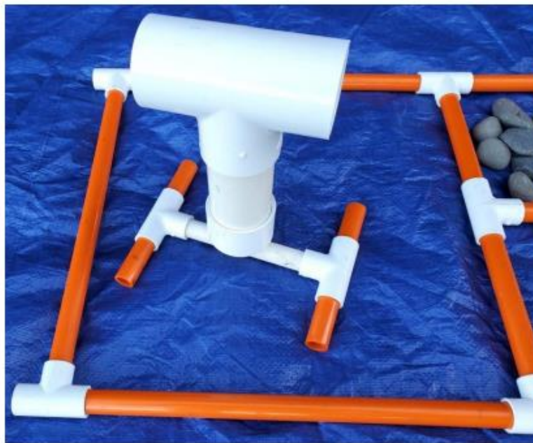
The designated area for the ADCP with the sediment area attached. The designated area is constructed from 1/2-inch PVC pipe.
