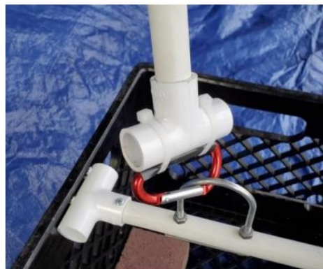
The MATE ROV Competition provided recovery line attached to the #310 U-bolt bale on the multi-function node.
