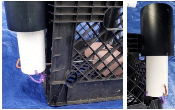
Left: The pin holding the recovery float. The recovery float rope is stored inside the float, above the pin. The pin passes through a loop in the rope, holding the rope in place until the pin is removed. Right: Two notches drilled into the bottom of the recovery float hold the pin in place.
